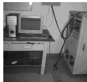
Fig. 4 The battery test system
